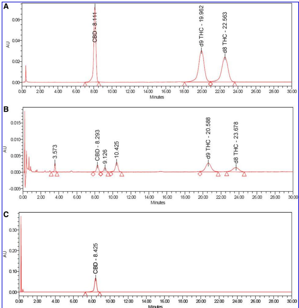
**FIG. 2.** UPLC-UV chromatograms in working standard (A), SGF at 75 min (B), HEPES at 360 min (C). UPLC, ultra-performance liquid chromatography; HEPES, 4-(2-hydroxyethyl)-1-piperazineethanesulfonic acid.
